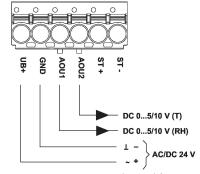
Connectors ST+ / ST- are only used for sensor types which additionally have a passive resistance sensor element for temperature measurement.
